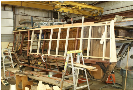
Down to the metal frame as the wood gets replaced where needed.
