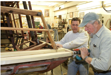
Down to the metal frame as the wood gets replaced where needed.
